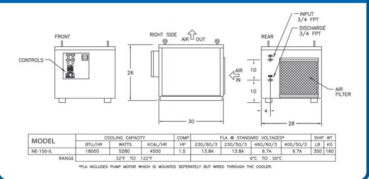
The In-Line Cooler cools fluid that is being pumped through it from a separate coolant tank. The digital temperature controller works to maintain the coolant temperature within 0.5° of set-point. The thermister sensor is mounted in the input line and is effectively sensing the sump coolant temperature. A circulating pump is mounted on the coolant tank. The NE-150-IL cooler will cool both water-based and oil-based coolants. The circulating coolant, however, must be clean.
